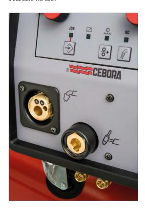
Second gas connection and additional dedicated solenoid valve when using the power source in TIG process.
