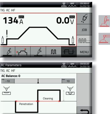
WIN TIG AC-DC 270 T is a three-phase power source with inverter technology for TIG (pulsed) and trode (MMA) AC DC welding, with built-in HF ignition. Comes with trolley for transportation of the power source. Can be connected to the optional cooling unit. wireless and to the auto (art. 1683) darken-(art. 434-optional) for protection mask. ing filter
